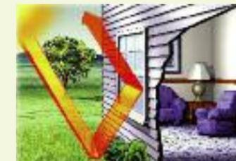
Low-E glass filters long-wave radiation from the sun. This reduces heat gain in the summer, keeping your home cooler.
